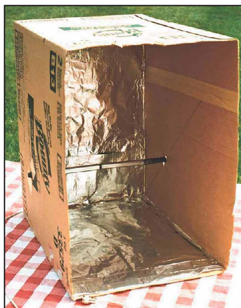
Figure 9—The completed simple uplink corner reflector.
